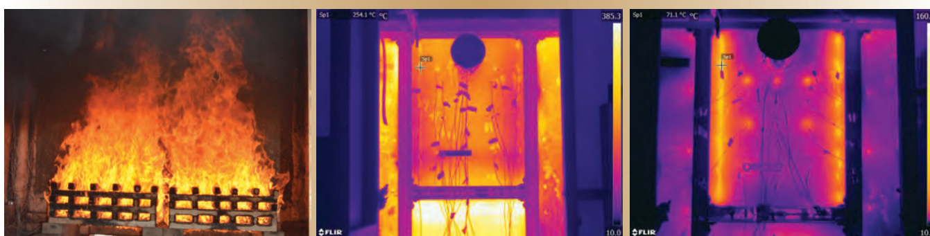
Fire at 10 minutes Ceiling temp: 290°C (550°F)
