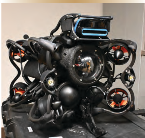
Oceanbotics™ SRV-8 remotely operated vehicle.
