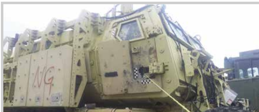
Damaged MRAP veh with EFP charge, Red River Army Depot, Texarkana, TX. The rope designates the trajectory (potential flight path) of the projectile. From an analysts perspective they can possible determine what triggers the device and what the enemy is aiming to achieve.
