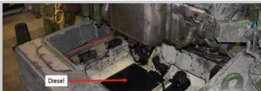
Maintenance personnel remove a Leo II power pack during a fire investigation. Note fuel staining on the side of the pack and fuel accumulation in the bottom of the engine compartment.
