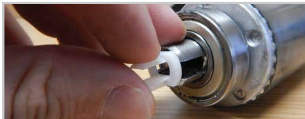
An incorrect fuel pump part was sent as a replacement for one supporting a heater being used for exercise. Due to a shortage of heaters, it was decided to attempt an in house print in order to create the part needed, and return the heater to service the same day.
