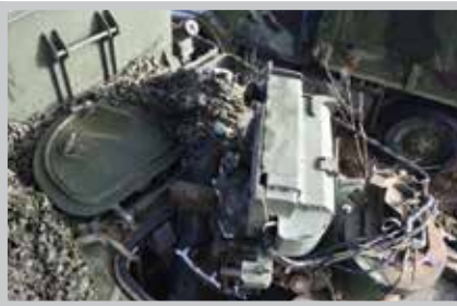
(Left) Engineering Variant LAV 6.0 following recovery from rollover site. (Right) Remote Weapon System was torn from mount and jammed into hatch.
