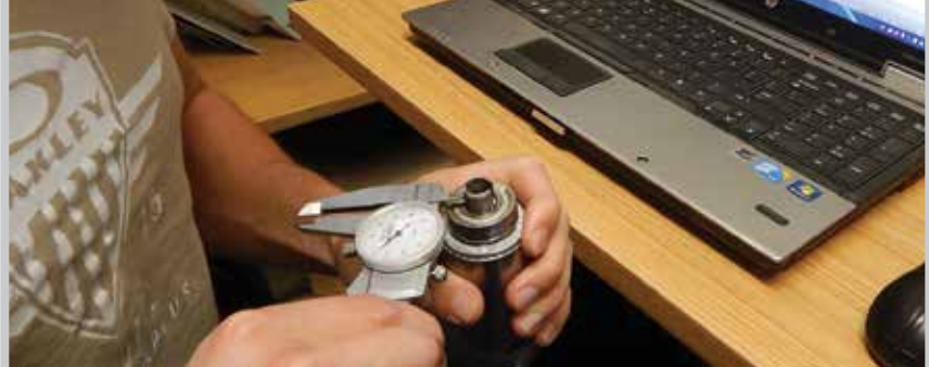
Designing the part took one hour with emphasis placed on measurements (fuel pump spindle and fan motor flutes). From these measurements, two Solidworks designs were created – one similar to the OEM part, and one redesign* that added durability.
