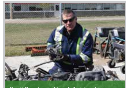
Scott Beeston holds a failed fan drive, believed to be causal to a U.S. Army HMMWV vehicle fire.
