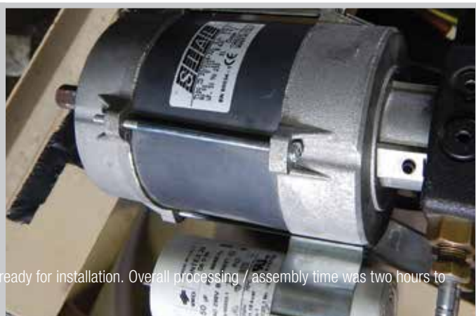
Final images show the printed part reassembled, and the fuel pump ready for installation. Overall processing / assembly time was two hours to return equipment's serviceability.
