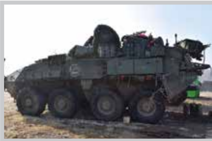
(Left) Engineering Variant LAV 6.0 following recovery from rollover site. (Right) Remote Weapon System was torn from mount and jammed into hatch.
