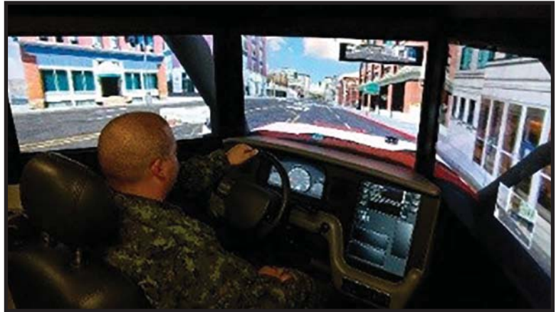
QL3 student using the CFMPA driving simulator. The CFMPA driving simulators are judgemental trainer tools used to help MP members in training develop the appropriate judgemental skills as they apply to driving in a policing context. They also ensure that candidates are able to comply with MP driving policies, procedures and orders appropriately and assist in learning articulation skills.
