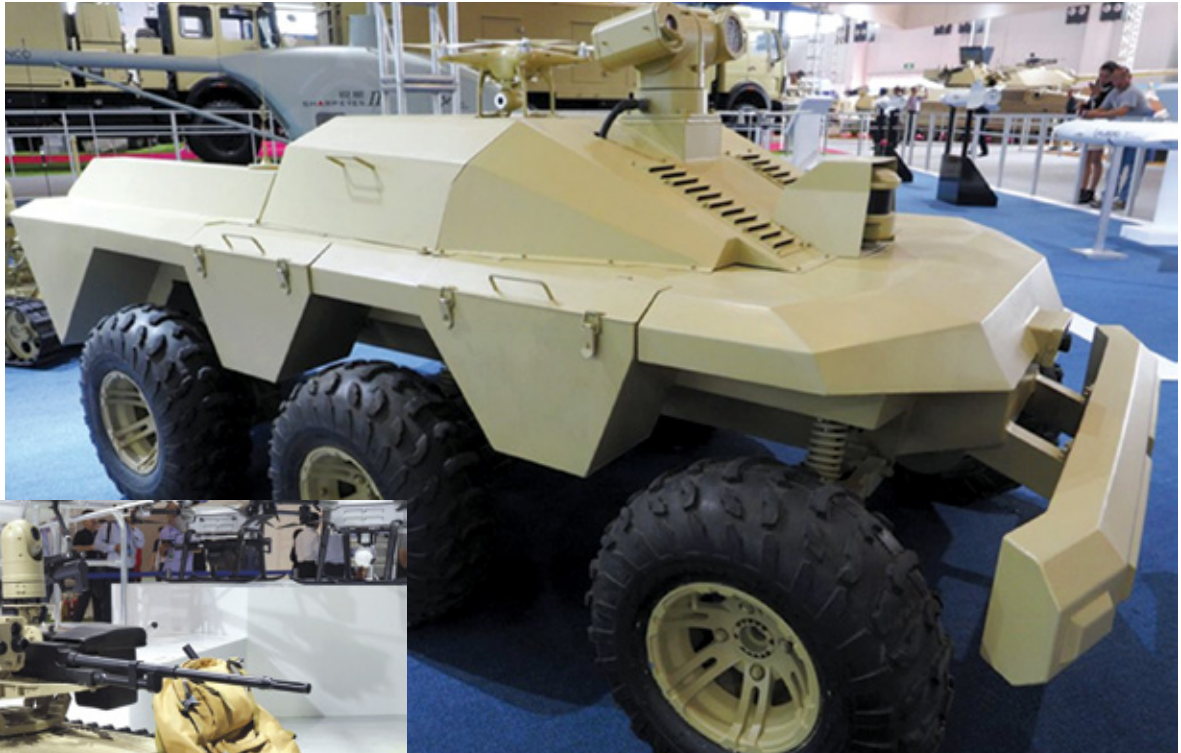
The Sharp Claw II Chinese 6x6 uncrewed ground vehicle is designed for a variety of roles, including reconnaissance, surveillance, combat engineering support, logistics and combat.
