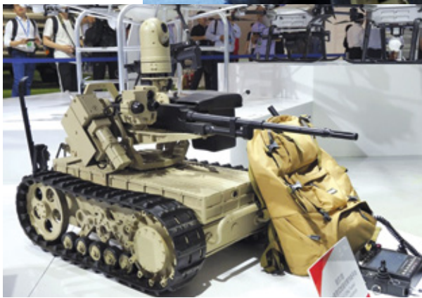
Sharp Claw I is a small, tracked scout robot designed to be carried in the cargo bay of the larger Sharp Claw II.
