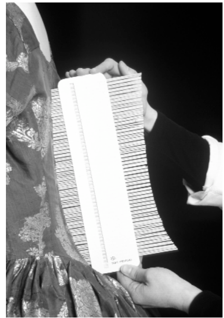
Figure 2. The soft profile gauge is used to measure the correct angle of the damaged baleen boning on this 18th-century silk robe.
