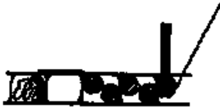
Figure 5c. The twill tape is woven between two applicator sticks per flute. The starting order is important. Begin the stick weave as shown here (*): under , then over ; not over , then under .
