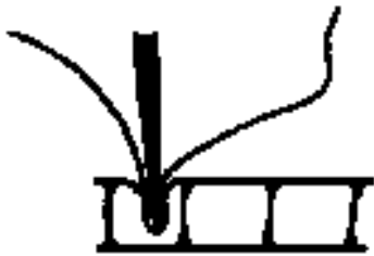
Figure 5a. The twill tape is inserted into the slit using a sharpened Popsicle stick.
