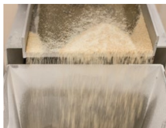
Allis-Chalmers Laboratory mill and purifier for durum wheat milling ►
