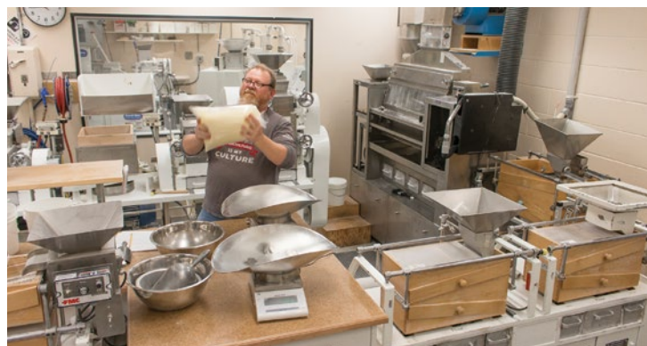
Allis-Chalmers Laboratory mill and purifier for durum wheat milling ►
