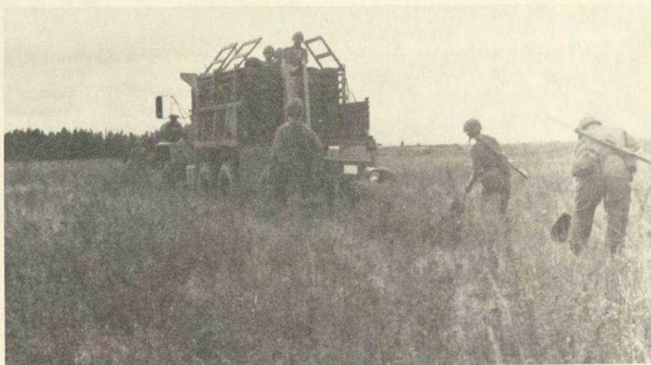
The obstacle sappers' minelaying — speed essential, concealment of lesser importance
