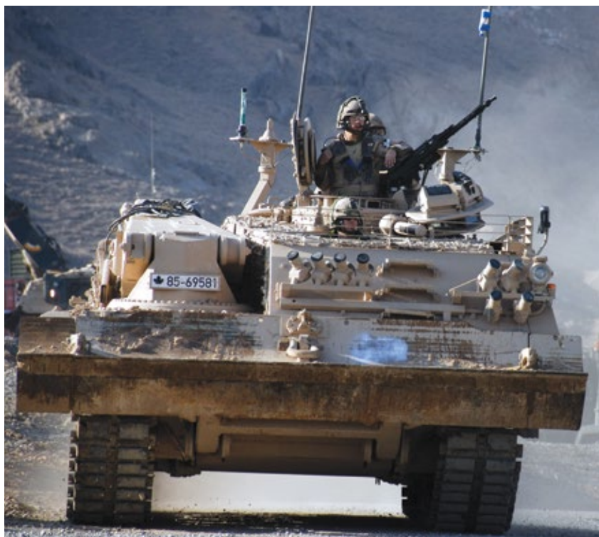
A heavy armoured recovery vehicle within the confines of a strongpoint near Panjwayi preparing to move as part of a convoy. This vehicle type is designed for recovering the new Leopard 2 tanks.
