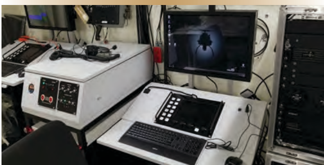
Figure 8. The temporary V-200 control station installed in the CSE technician office aboard a frigate.
