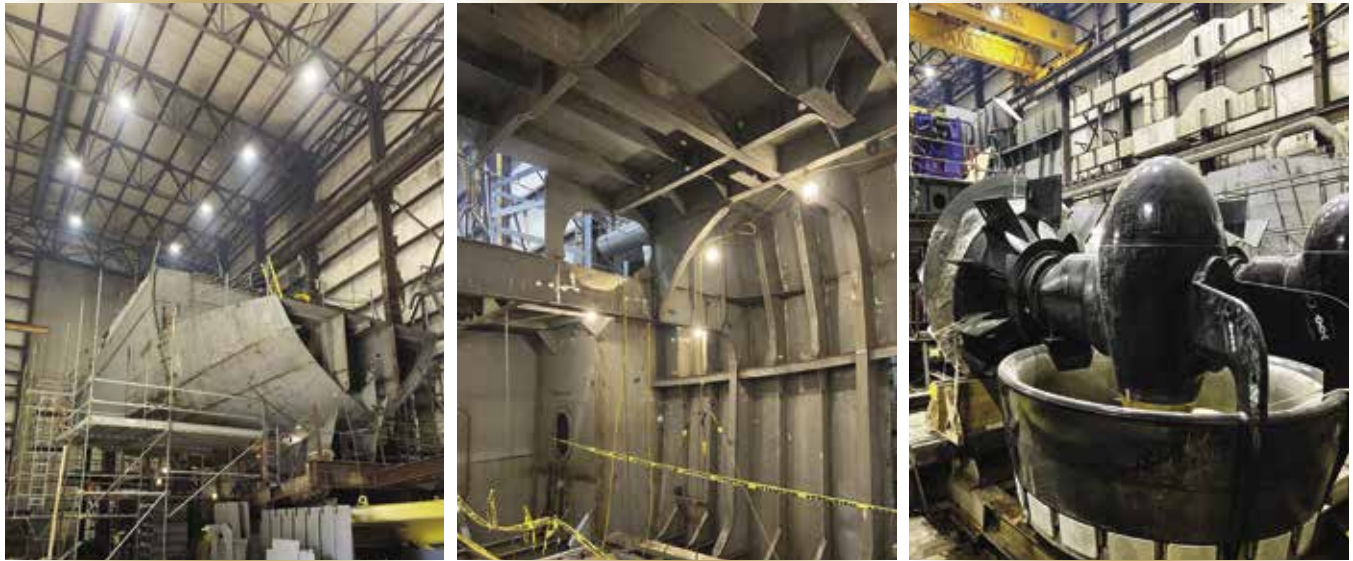
Figure 5. The first NLT (Hull 228) takes shape at left, with an interior view of the engine room at centre, and an azimuthing stern-drive unit waiting to be installed at right.
