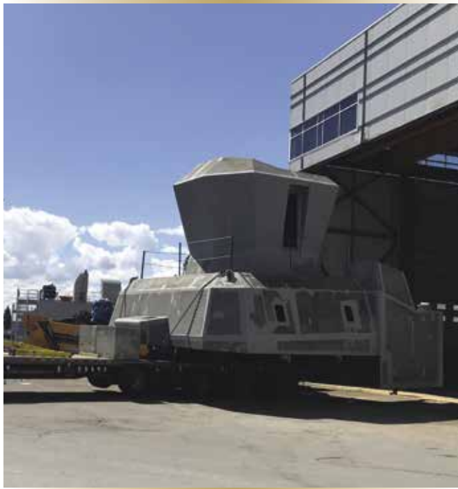
Figure 4. Superstructure assembled at the Industries Océan facility in Québec City is moved out of the construction hall for water transport 120 km down the St. Lawrence River to the Isle-aux-Coudres shipyard.
