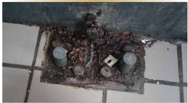
Figure 6. A severely corroded galley appliances connection.
