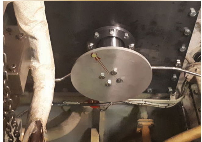
Figure 1. Gear shaft extension stub with radial orientation marking to help determine the source of the noise.
