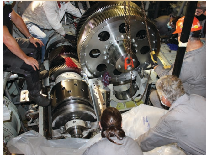
Figure 4. Formation gearing inspectors Patti Fraser and Stephane Chouinard observe the installation of the new gear.
