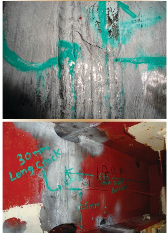
Figure 3. A 30-mm crack found on the web of a girder aboard HMCS Ville de Québec (FFH-332). (Huang, 2021)
