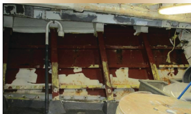
Figure 1. Area of corroded steelwork on the port side of the foc'sle mezzanine deck.
