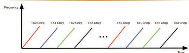
Figure 5. FMCW signal using TDM. TX indicates which T/R module is transmitting.
