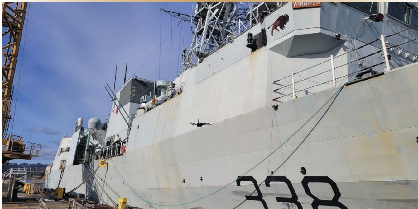
Figure 1. The Skydio X2D Remotely Piloted Aerial System (at centre of image) actively taking high-resolution 2D ship structure photos of HMCS Winnipeg last October.
