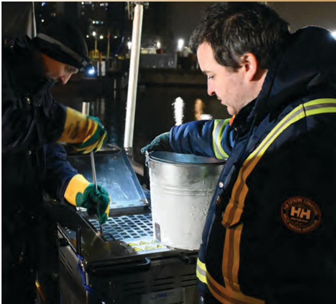
Technicians from the FMFCS Submarine Electrical shop prepare the dry-ice pellets (right) in the open air, jetty-side.
