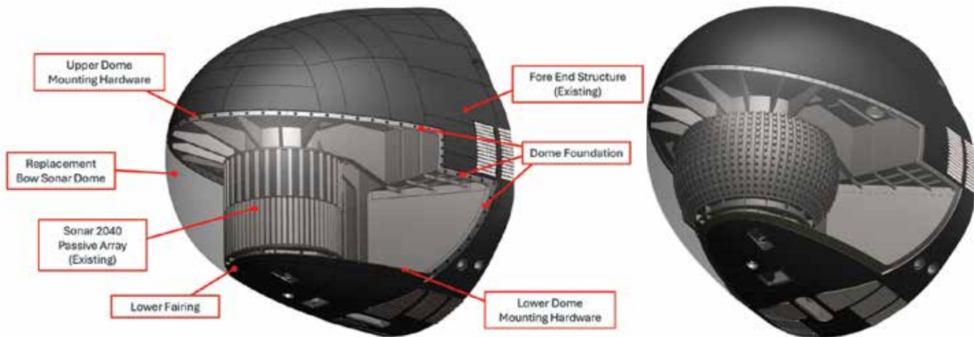
Comparison of the legacy 2040 array (left) to the new VCBA (right).
