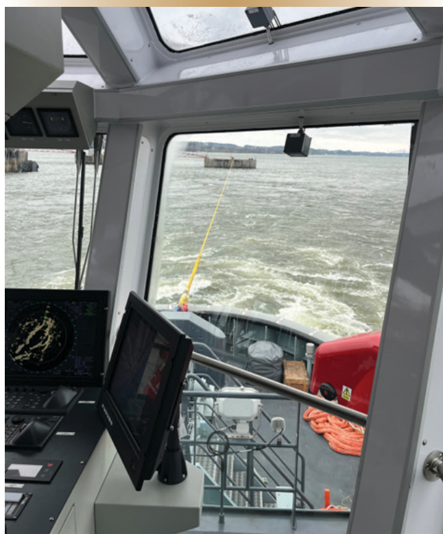
Bollard pull trial on CFAV Canso .
