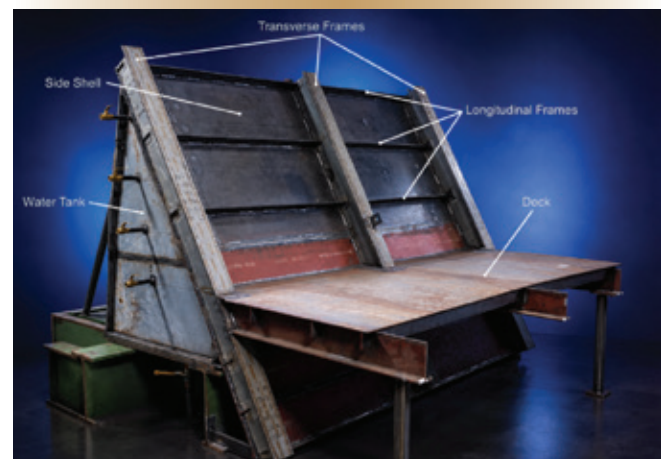
Figure 1. To-Scale Ship Structure Test Rig
