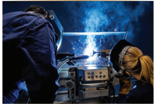
Figure 3. Instrumented Weld Trials on Test Rig
