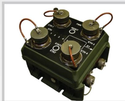
The LESv2 acts as a network switch within the ELAN and provides additional connectivity to Ethernet attached equipment. The LESv2 is connected to the ELAN ring in the same way as the CSBs in a platform, and provides eight additional Ethernet ports.
