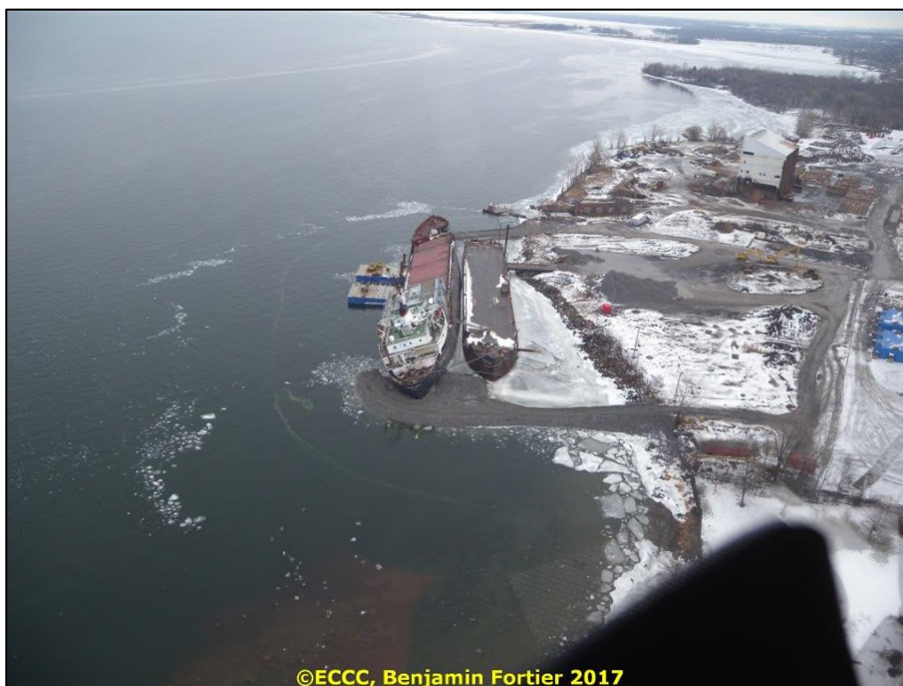
Figure 3-14: Bubble curtain deployment on the St. Lawrence River (courtesy of ECCC).
