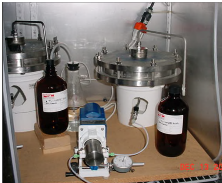
Figure 4-5: Thin-layer column leaching test (Blasland, Bouck & Lee Inc. et al. 2006; Brannon et al. 1994).
