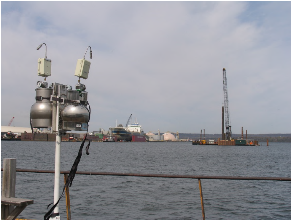
Figure CS4-4: Suma canisters used as part of the air monitoring program during the project (courtesy of ECCC).
