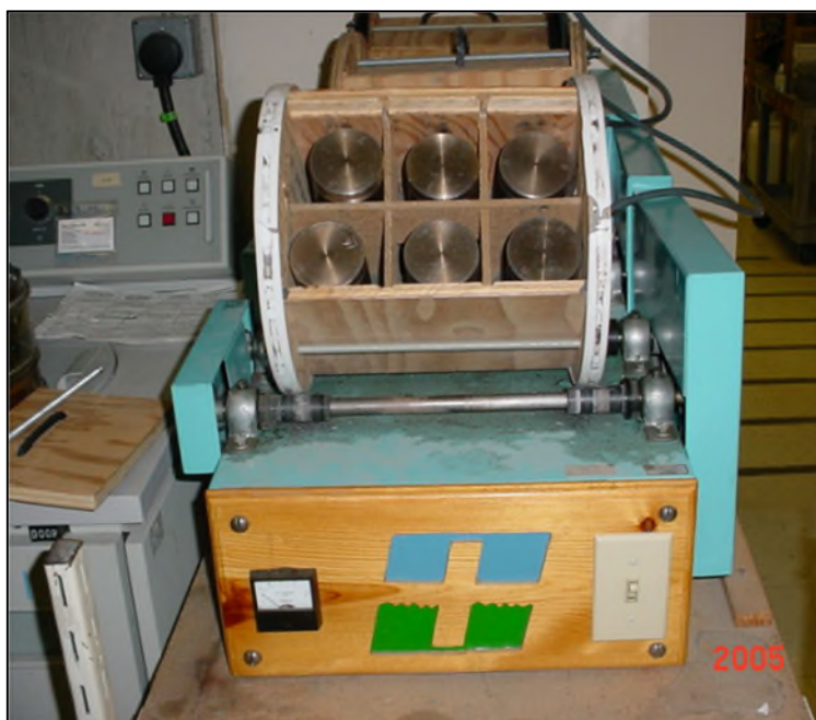
Figure 4-6: Sequential batch media adsorption test. (Blasland, Bouck & Lee Inc. et al. 2006)
