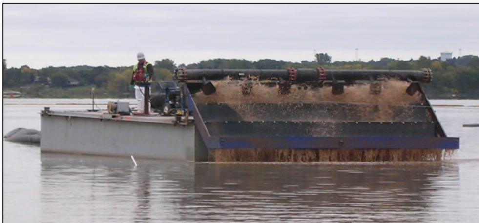
Figure 5-13: Angled-plate hydraulic spreader barge operating at the Fox River site, Wisconsin (courtesy of M. Palermo and C. Vogt).
