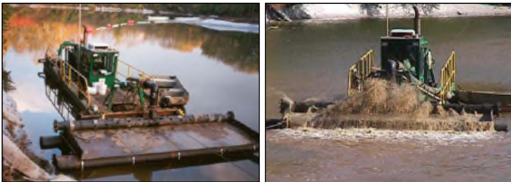
Figure 5-12: Flat-pan spreader barge used at Mock's Pond, Indiana (courtesy of M. Palermo and C. Vogt).
