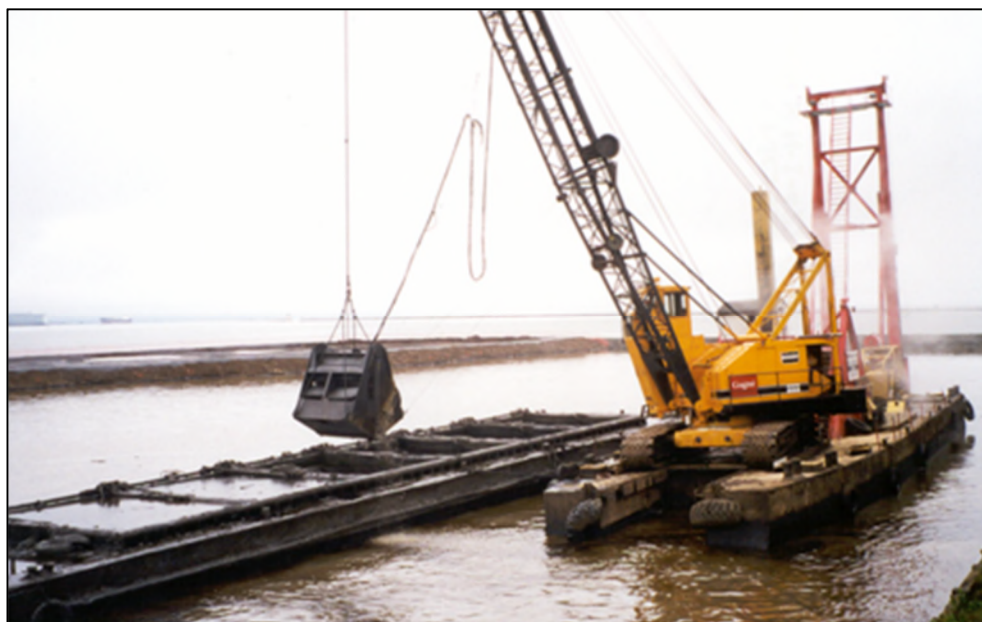
Figure 3-4: Mechanical dredge with scow (courtesy of ECCC).
