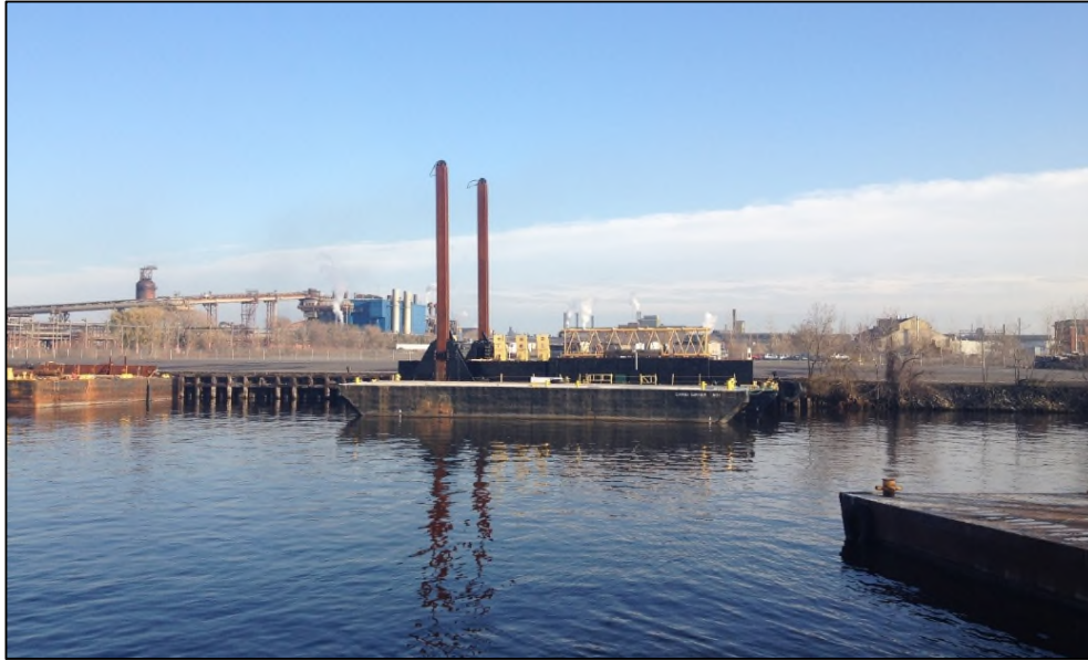
Figure 3-5: Work barge with raised spuds and anchoring system (courtesy of ECCC).
