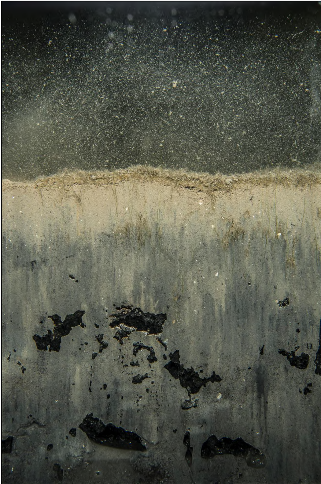
Figure 5-3: SPL camera image showing the water, the sediment/water interface, and the sediment (courtesy of Fisheries and Oceans Canada).
