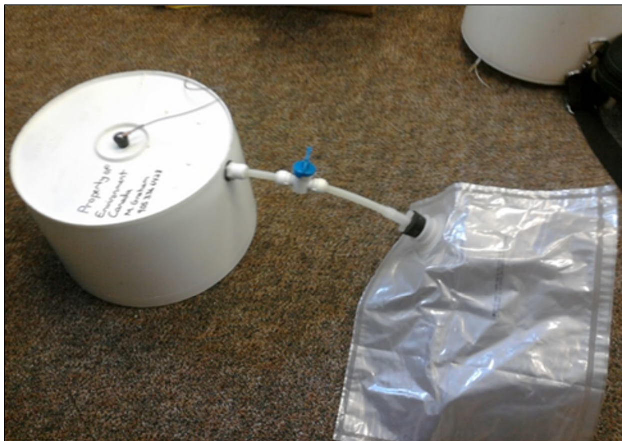
Figure 5-4: A seepage meter of Environment and Climate Change Canada (courtesy of ECCC).
