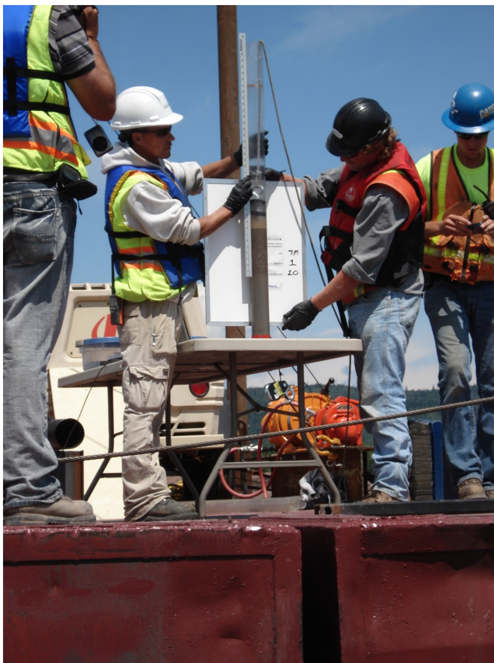
Figure CS2-7: Cap thickness verification via cores (courtesy of AECOM).
