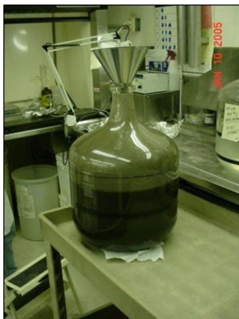
Figure 4-6: Sequential batch media adsorption test. (Blasland, Bouck & Lee Inc. et al. 2006)
