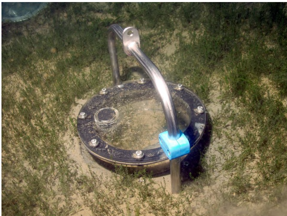
Figure 5-9: A core sample for use in the circular flume of Environment and Climate Change Canada (courtesy of ECCC).
