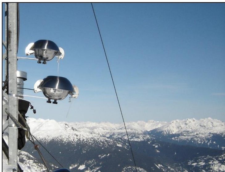
Figure 3 - Two passive samplers used in the Global Atmospheric Passive Sample (GAPS) Megacities project, located at a background site on top of a mountain in Whistler, British Columbia. The samplers are located high in the air attached to a metal frame, in order to collect air particles on a polyurethane foam disk. The disks are contained in metal traps designed using two metal bowl-like structures fastened together with a small space in between to allow air circulation.
