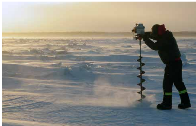
ECCC hydrometric technologist drills on the frozen McKenzie River to measure water flow under ice.
