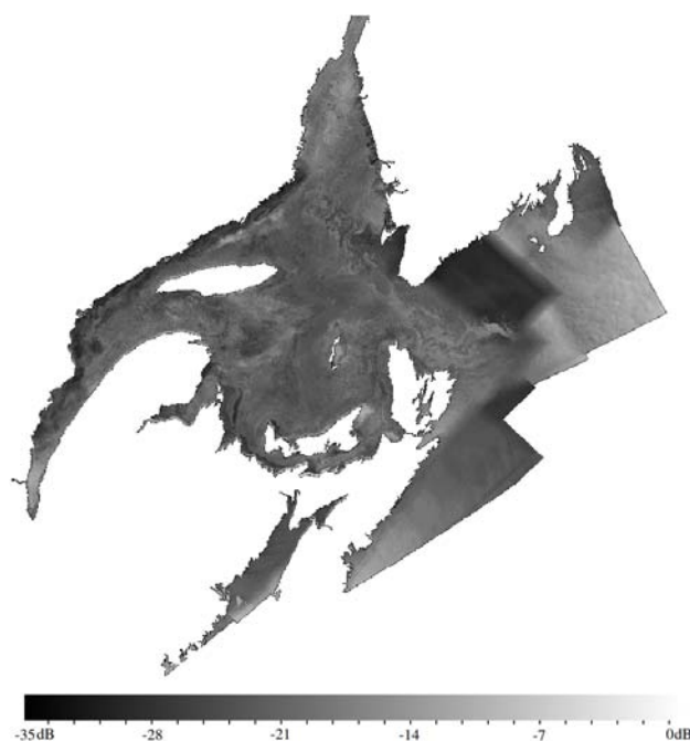
Fig. 6. An example of a SAR mosaic (based on RADARSAT-2 data, © MDA), on 5 March 2009; the boundaries between SAR frames have been smoothed in the mosaic. The white areas are either land or sea areas not covered by the SAR data. The scale in dB is shown by the color bar.
