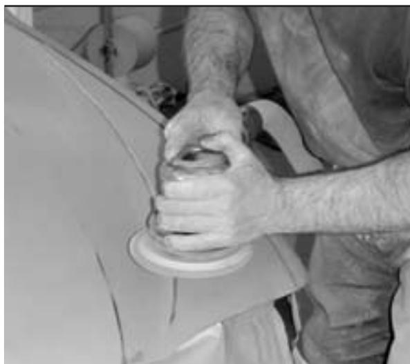
Sand the surface before applying paint stripper.
