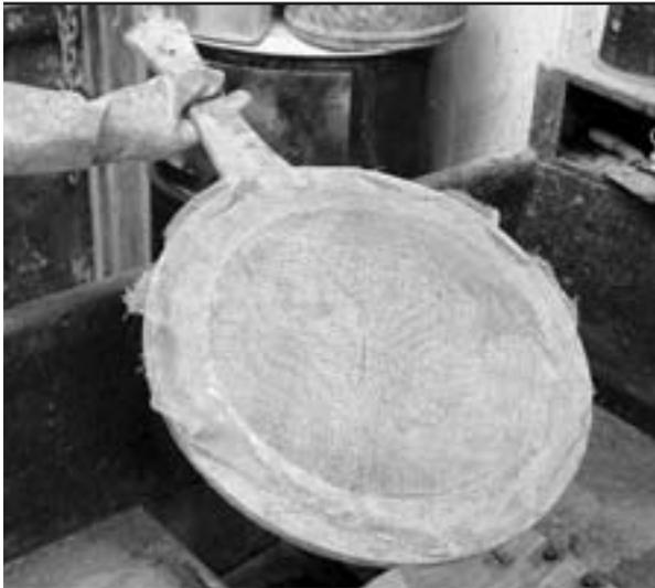
Remove paint chips from used paint stripper with a strainer.
