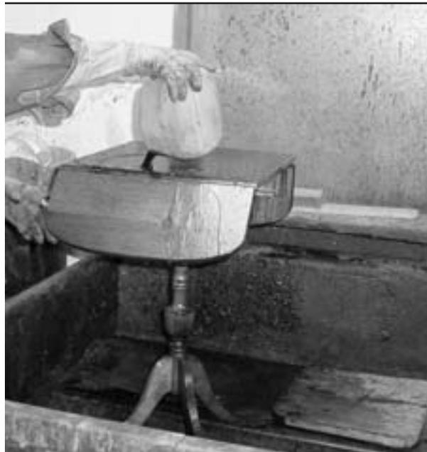
Capture and reuse paint stripper, if possible.
