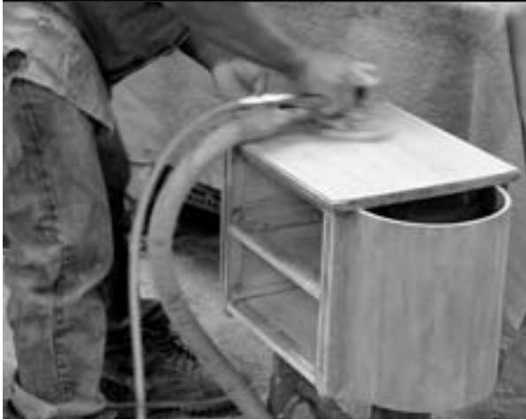
Strip excess coats of paint with sandpaper before applying the paint stripper.
