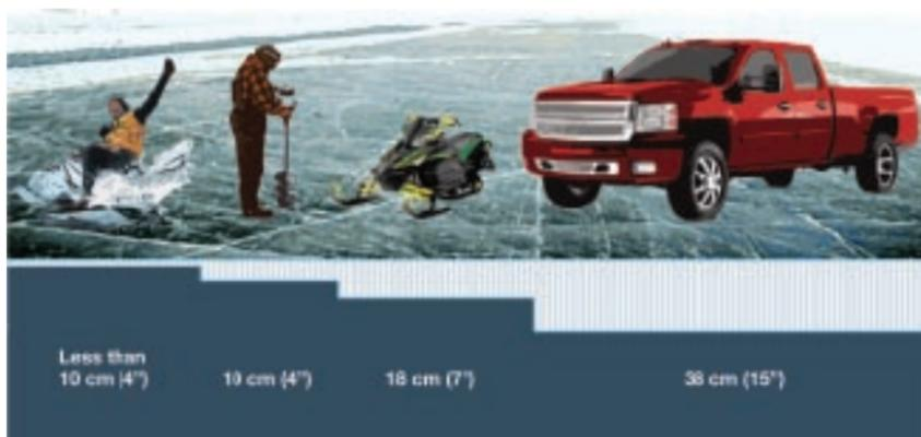
*Minimum ice thicknesses for parked or slow moving loads less than 2 hours. For heavier vehicles, refer to the Best Practice and your Ice Safety Plan.*
