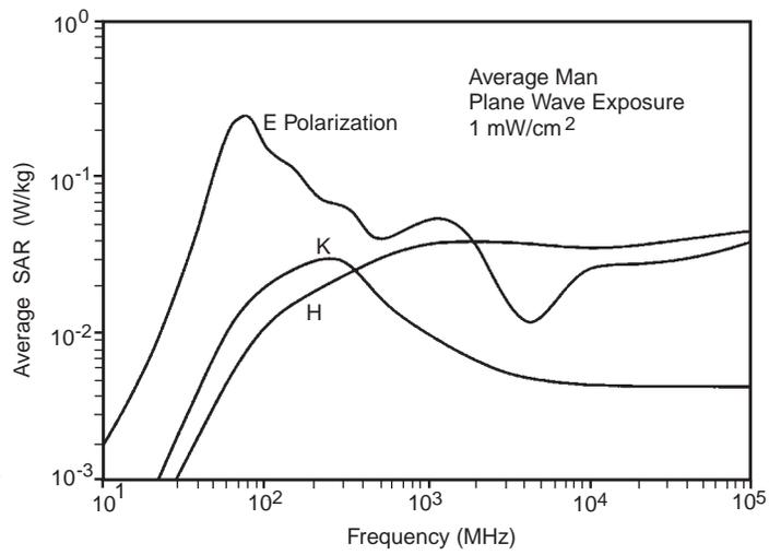
Figure 1 – Average specific absorption rate for an average man exposed to 1 mW/cm<sup>2</sup> plane wave. E polarization denotes the electric field parallel to the body, H denotes the magnetic field parallel to the body and K denotes the wave moving from head to toes or toes to head.
