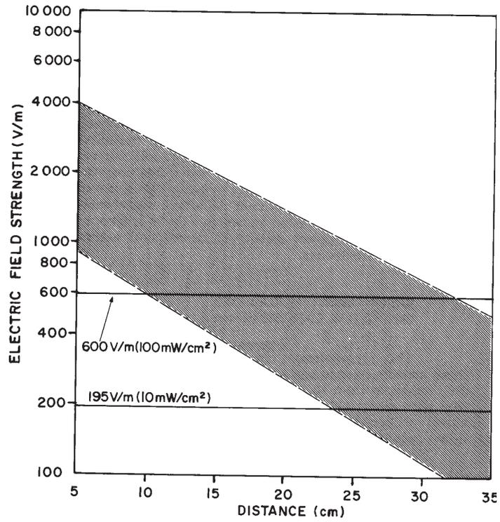
Figure 2b – The range (shaded area) of the electric field intensities around cables of the short-wave diathermy device for various types of electrodes and typical power settings.
