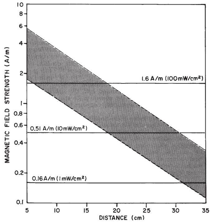
Figure 2a – The range (shaded area) of the magnetic field intensities around cables of the short-wave diathermy device for various types of electrodes and typical power settings.
