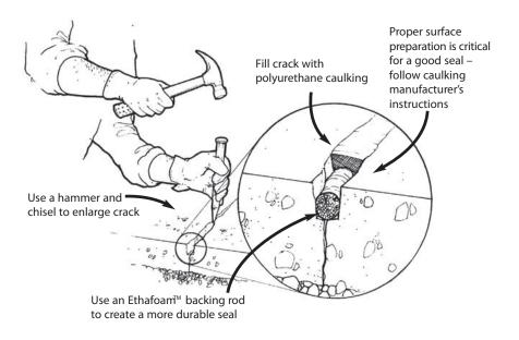
Figure 5  $_{\uparrow}$  Sealing foundation wall and floor cracks.
