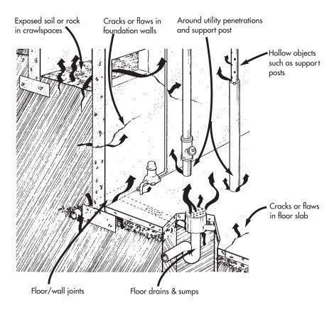
Figure 1  $_{\uparrow}$  Typical radon entry routes in poured concrete foundation walls and floors.
