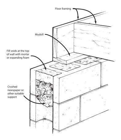
Figure 4  $_{\uparrow}$  Sealing voids in the top of concrete block walls.
