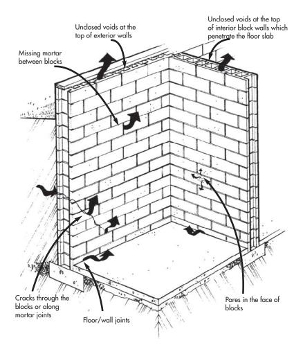
Figure 2  $_{\uparrow}$  Typical radon entry routes in concrete block foundation walls.
