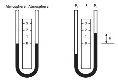
Figure 7 † U-tube manometer.
