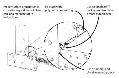
Figure 3 1 Sealing foundation wall and basement floor joint.
