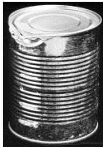
Dented at junction of side and end
