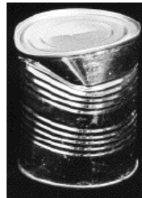
Sharp dent or dent on seam
