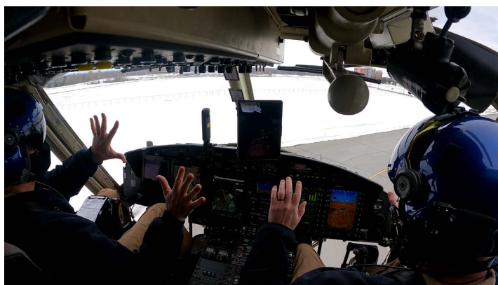
Cockpit view of the NRC's Bell 412 Advanced Systems Research Aircraft with test pilots supervising the autonomous landing in between obstacles.
