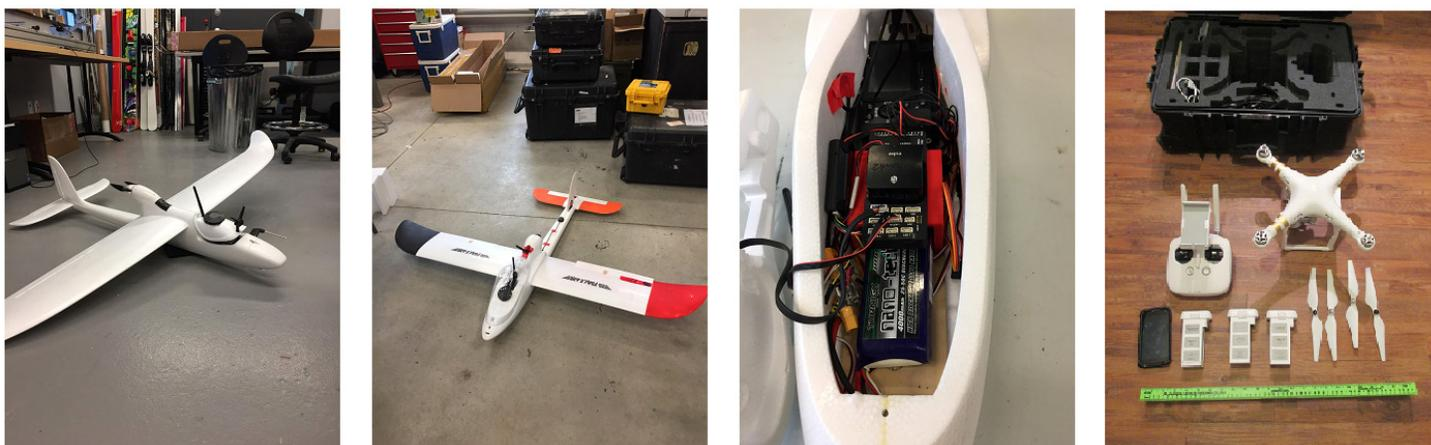
Figure 5: From left to right: the BlitzRCWorks Skysurfer Pro, Finwing Penguin, interior of the Finwing Penguin, and the DJI Phantom 3 Professional.
