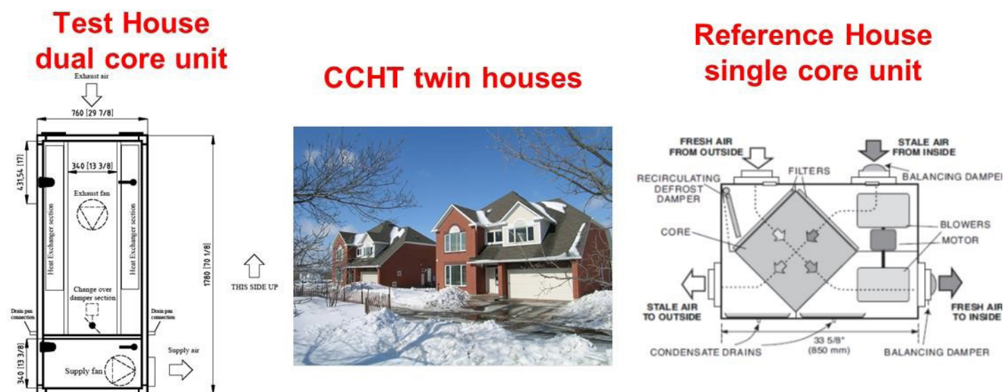
Figure 3: Side-by-side testing using the Canadian Centre for Housing Technology (CCHT) twin research houses.
