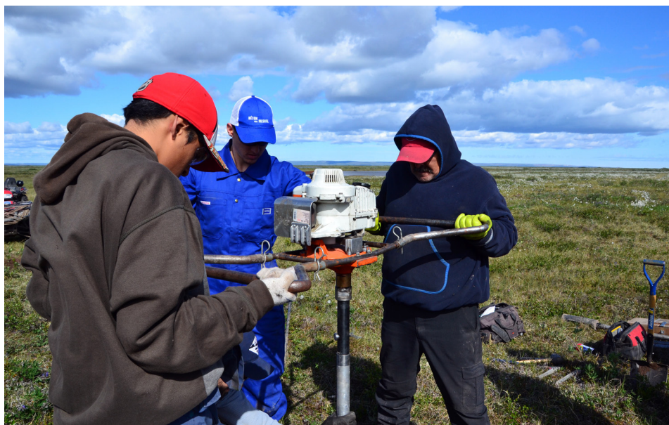
Researchers, including Kugluktuk youth and park staff, operate a portable earth auger to sample permafrost: POLAR
