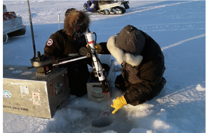
Tommy Epakohak (left) and Ryan Angohiatok pull a CTD instrument up from the ice during CROW 2020 near Finlayson Islands: Mike Dempsey
