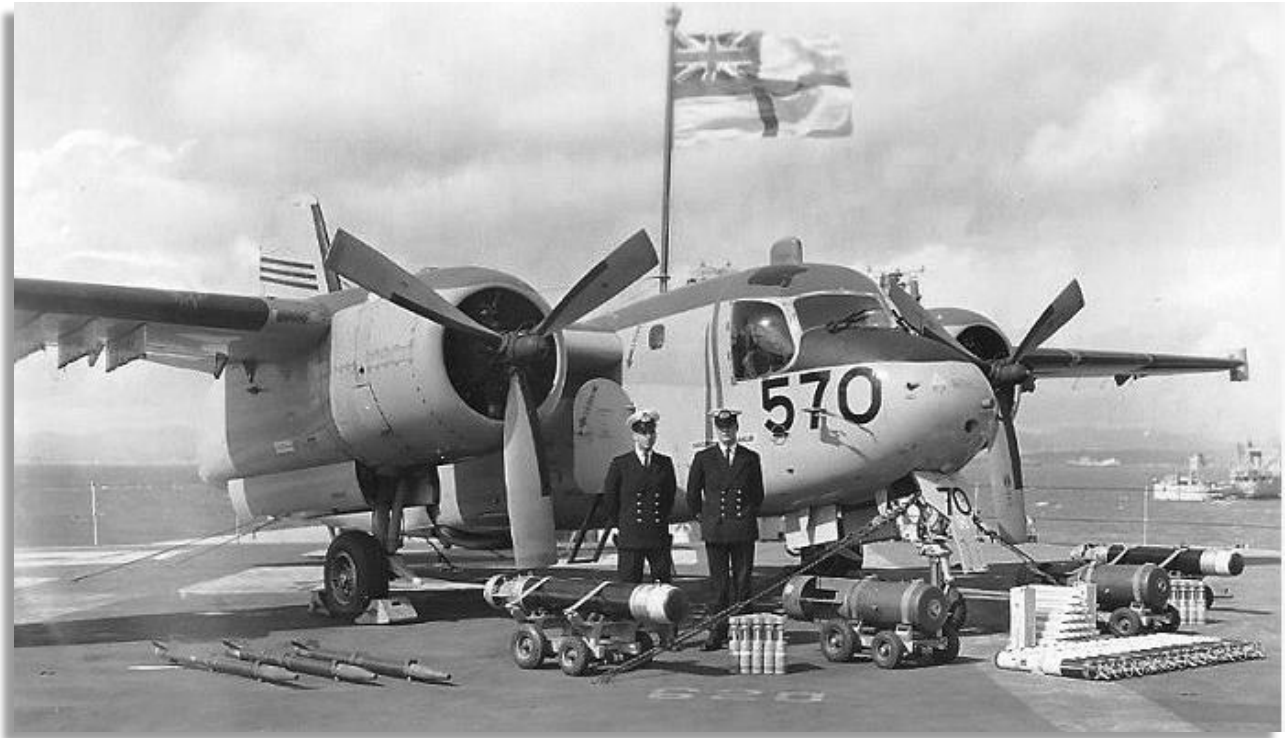
De Havilland CS2F Trackers of naval air squadron VS-880 carried out surveillance missions from shore bases and HMCS Bonaventure. Here we see the array of anti-submarine weapons and sensors typically utilized by maritime patrol aircraft, including sonobuoys, air-to-surface rockets, depth bombs and A/S torpedoes. (DND)
