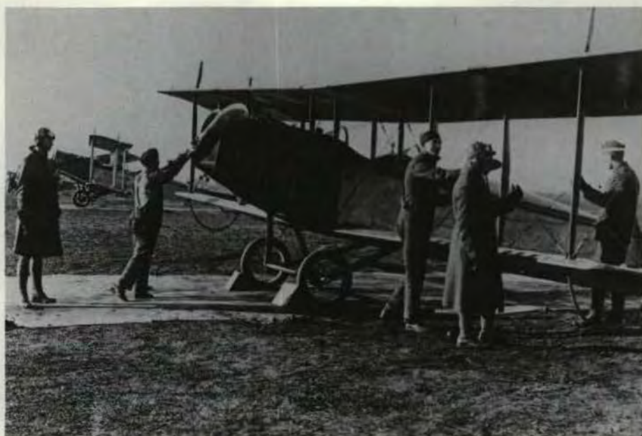
Pre-flight test of JN4 rigging by instructor, cadet, and ground crew (RE 19715)
