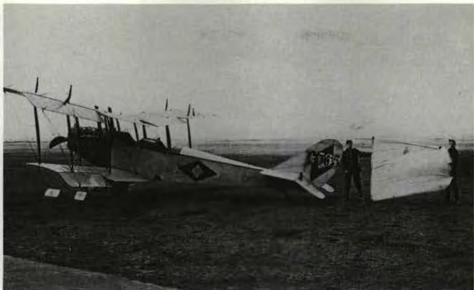
JN4a and drogue used for aerial machine-gun training at the School of Gunnery, Camp Borden. The drogue was towed further behind the aircraft than as demonstrated in this picture. (RE 20804-3)
