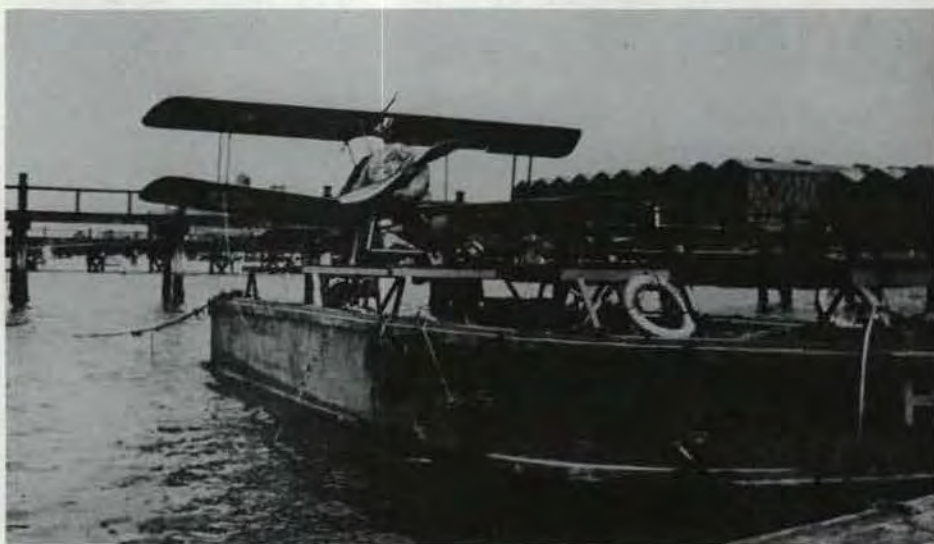
A Sopwith Camel aboard a lighter at Felixstowe. Towed into the wind at 30 knots by a destroyer, lighters like these provided an adequate take-off platform for the Camel. Landing, the aircraft either had to reach dry land or come down in the sea alongside the lighter. (Q 69367)
