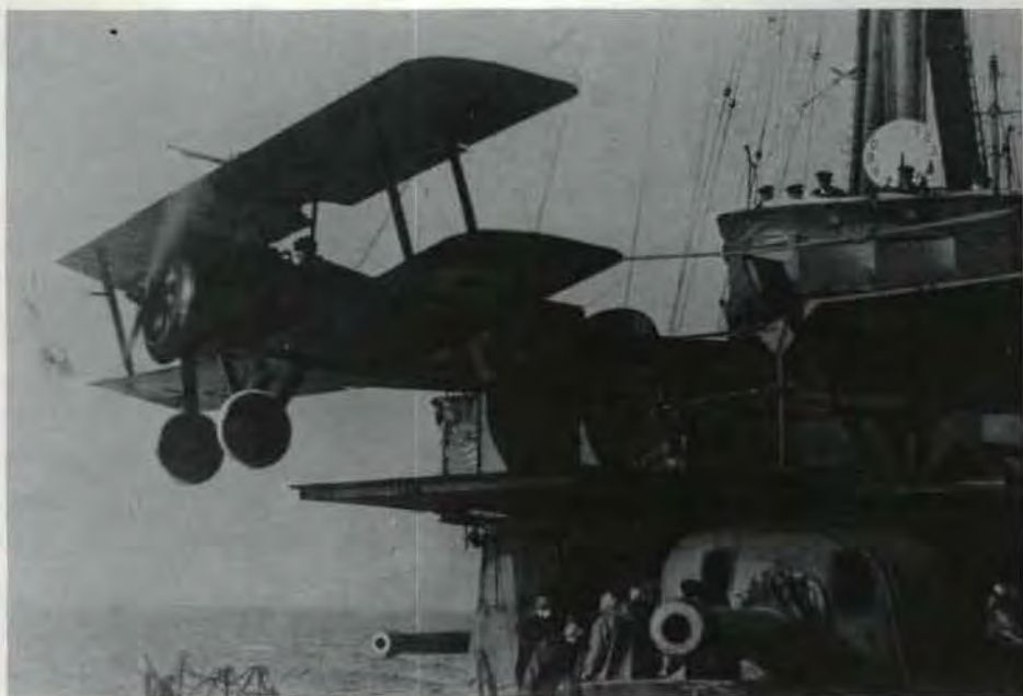
2/Lt W.S. Lockhart of Moncton, NB, flying a Sopwith Camel off the forward turret ramp of the light cruiser, HMAS Sydney , 1918. Machines launched in this manner either had to land on shore or 'pancake' into the sea beside the mother ship. (PMR 71-872)
