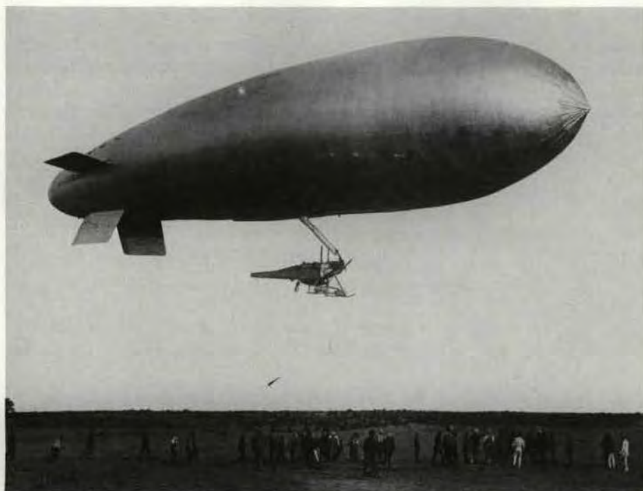
An early SS-type coastal airship returning to its base in the Aegean after a patrol over Gallipoli. The combined control car and engine gondola is simply the fuselage and power plant of a BE2c suspended beneath the gas bag. (Q 13498)
