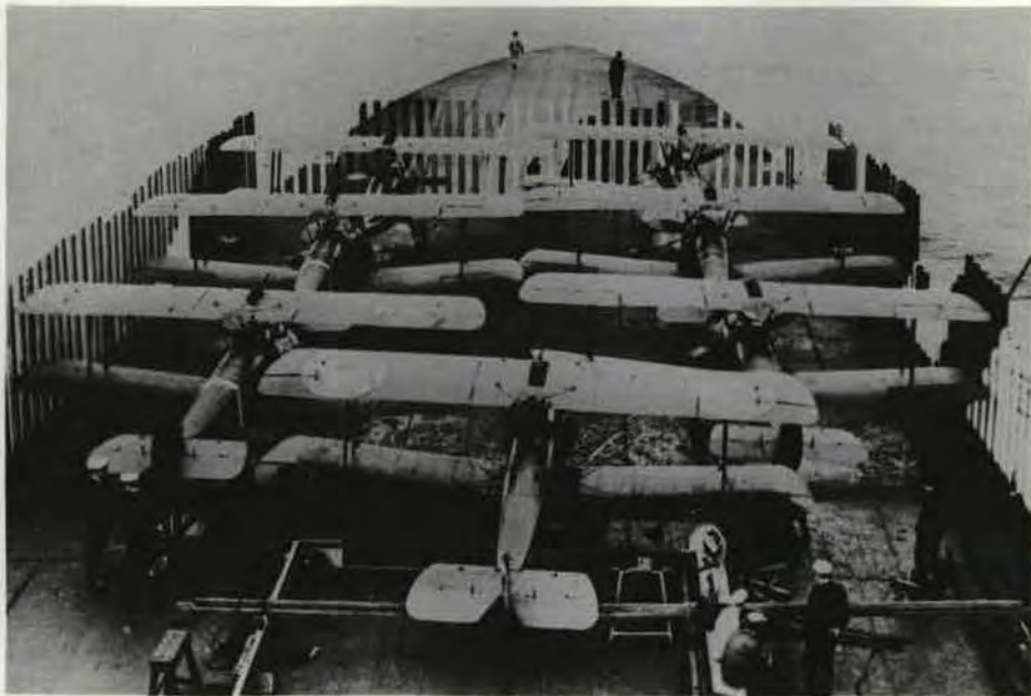
Sopwith Camels lined up on the 228-ft forward flight deck of HMS Furious . Originally a heavy cruiser, Furious was converted to an aircraft carrier by stages, a longer (280 ft) after flight deck being added later. (PA 6280)
