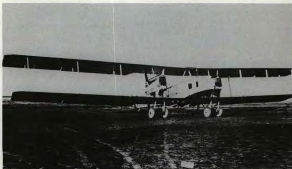
The Gotha G-V had an additional pair of wheels under the nose, to ease the stress of landing, and a 'tunnel' through the fuselage which permitted the rear gunner to fire downwards as well as laterally and upwards. (PMR 72-526)
