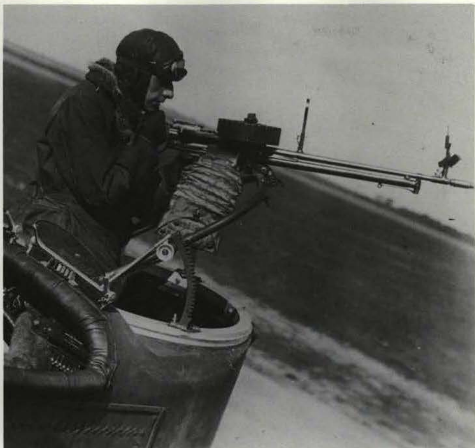
The nose of a Handley Page bomber. The drum on top of the Lewis gun is the magazine and the pouch below it, on the gunner's right, collected used casings and stopped them flying back in the pilot's face. (AH 530)
