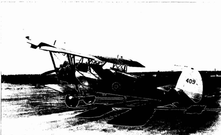
Until the Second World War the RCAF used the Armstrong Whitworth Atlas for its army co-operation role, particularly on militia summer manoeuvres. The bar and hook arrangement under the fuselage was used for snatching messages from the ground. (PA 063304)
