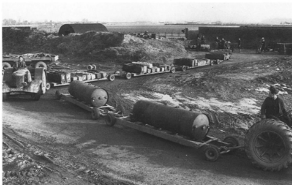
A particularly busy part of any bomber station before an operation was the bomb dump. The first tractor is towing two 4000-lb high-capacity bombs, while the second pulls a train loaded with incendiary containers. (PL 26964)
