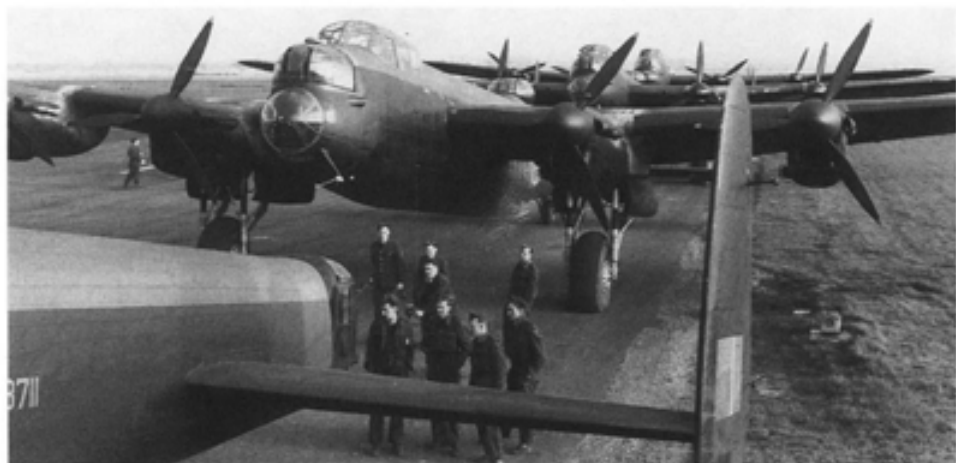
In March 1944 No 419 Squadron, based at Middleton St George, became the first to be equipped with the Canadian-built Lancaster X. This lineup shows the enlarged bomb-bay doors designed to allow these machines to carry an 8000-lb bomb. KB 711, whose tail can be seen in the foreground, was the first Lancaster X to be lost on operations, going down on the night of 1/2 May 1944 during a raid on the railway yards at St Ghislain, France. (PL 29474)
