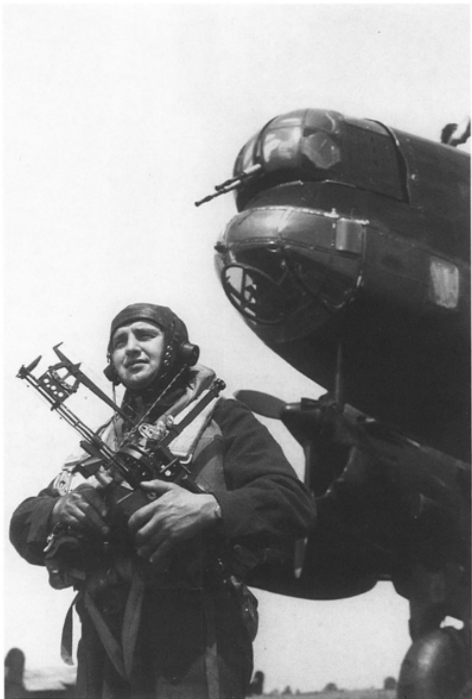
A bomb-aimer at a Heavy Conversion Unit holds a Mark IX Course Setting Bombsight used by Bomber Command in the early years of the war. (PL 19336)
