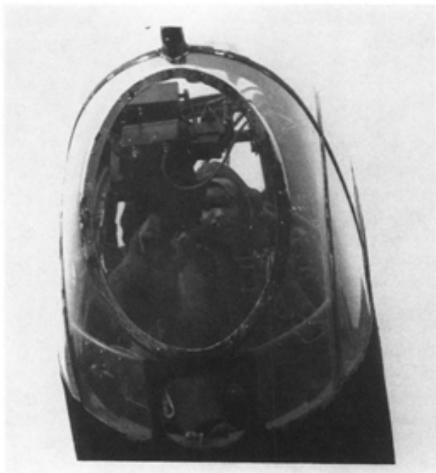
Until the separate trade of bomb-aimer was introduced, it was the task of the observer to ensure accurate bombing. This is the bomb-aiming position in a No 408 Squadron Hampden. (PL 4708)
