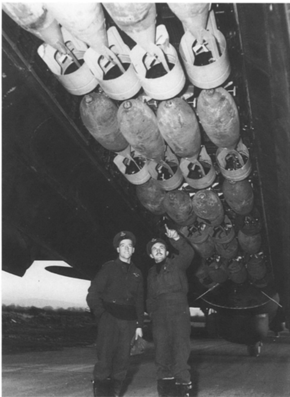
The pilot and bomb-aimer of a No 428 Squadron Lancaster X stand beneath the open bomb bay of their aircraft prior to an attack on an oil refinery in the Ruhr late in 1944. The comparatively short range to the target allowed a full load to be carried, in this case 500-lb general purpose high-explosive bombs. The dome of the H2S radar installation is visible immediately behind the bomb bay. (PL 40683)
