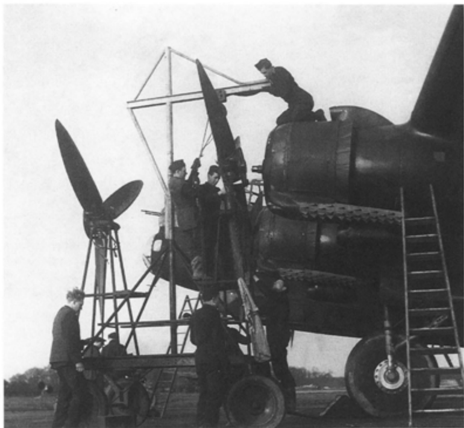
Groundcrew of No 426 Squadron engaged in changing the propellers on the Hercules engines of a Lancaster II. (PL 26008)
