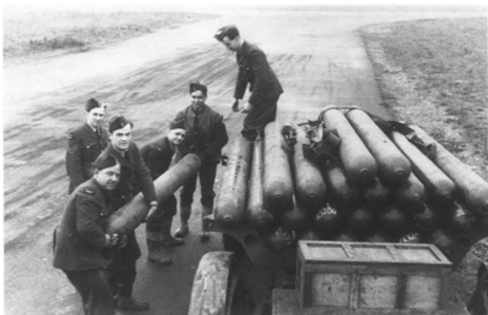
Oxygen was vitally important to Bomber Command aircrew. Here, groundcrew from No 434 Squadron are about to instal fresh oxygen cylinders in a Halifax in the fall of 1943. (PL 22425)
