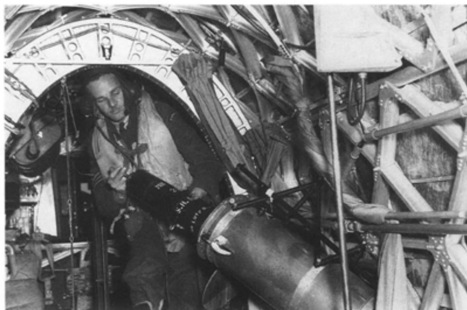
Using the flare chute in a Wellington. The distinctive fabric-covered, geodetic construction of the Wellington's fuselage is prominent. (PL 4661)
