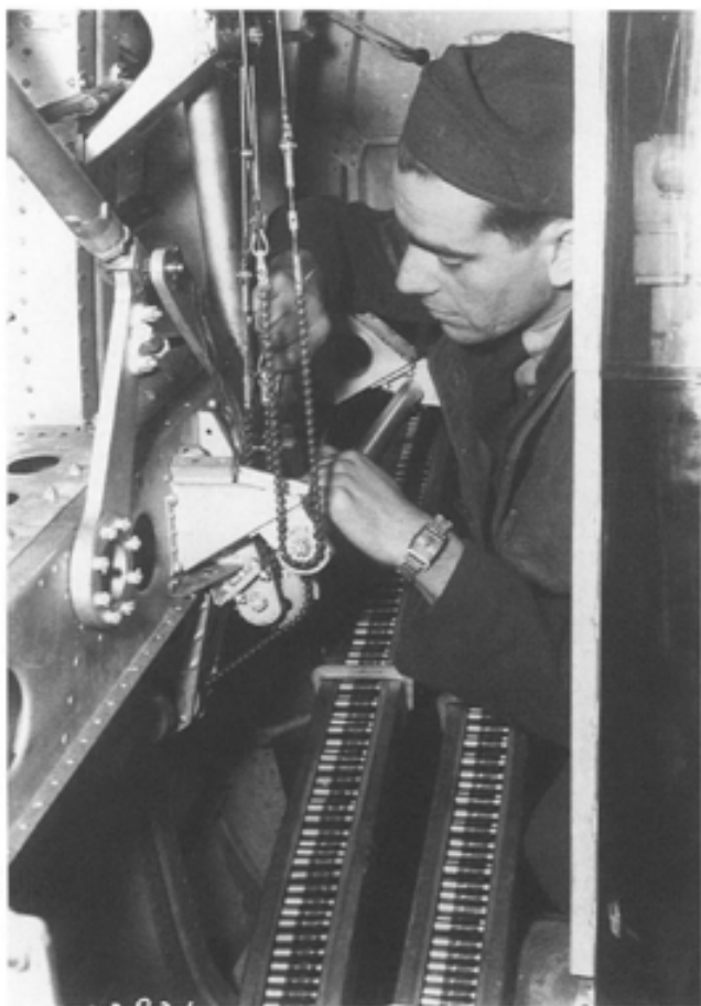
Leaning over the tracks supplying ammunition to the guns in the rear turret, a technician adjusts the elevator balance bars of a Halifax. (PL 22921)
