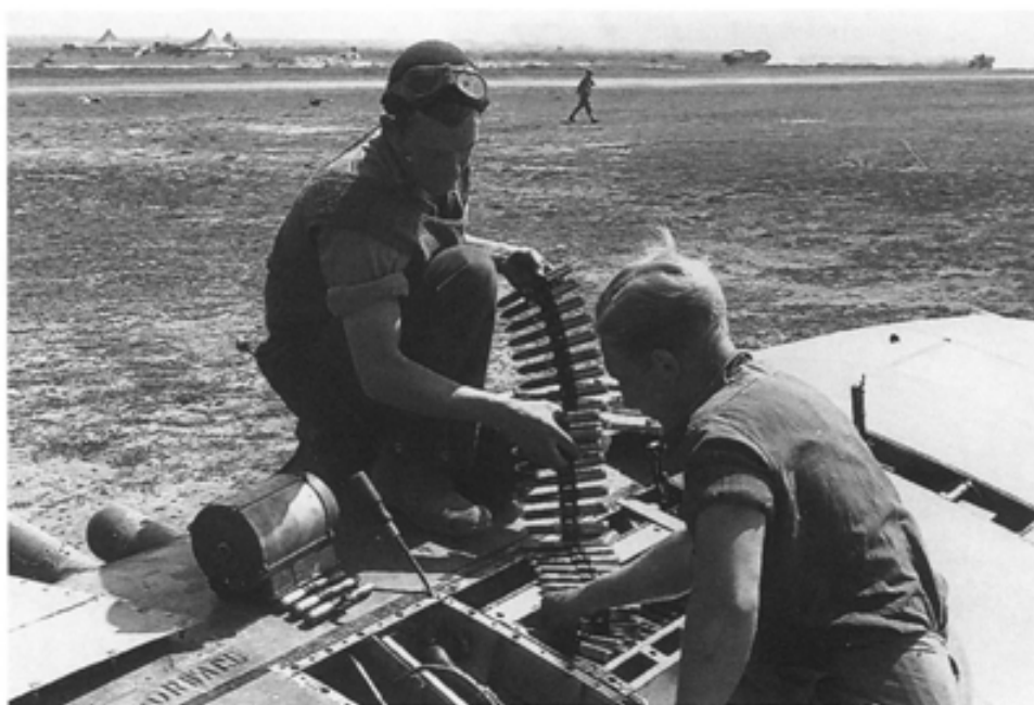
Arming the 20-millimetre Hispano cannon of a Spitfire. (PL 27501)
