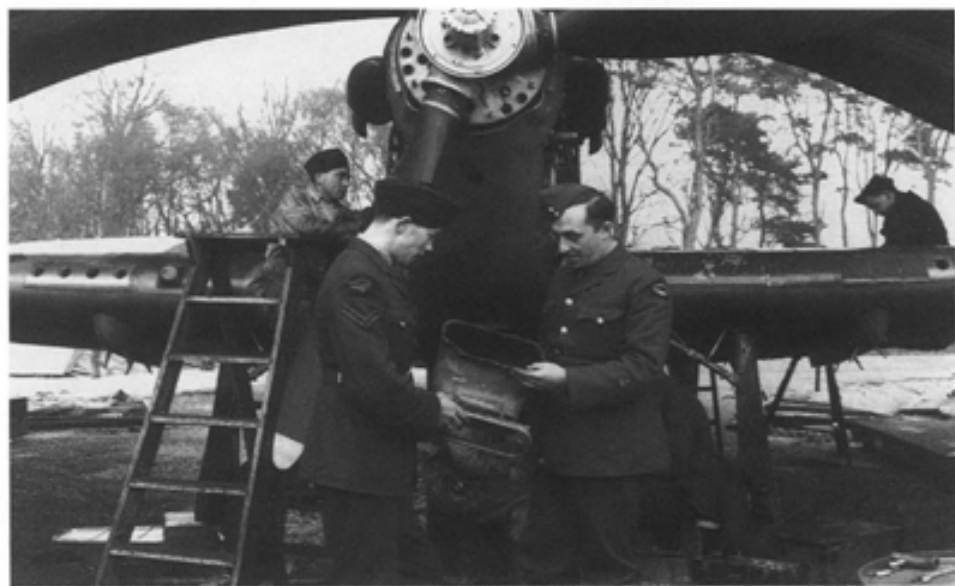
No 402 Squadron groundcrew inspect the carburettor air scoop of a Hurricane IIB. (PL 7121)
