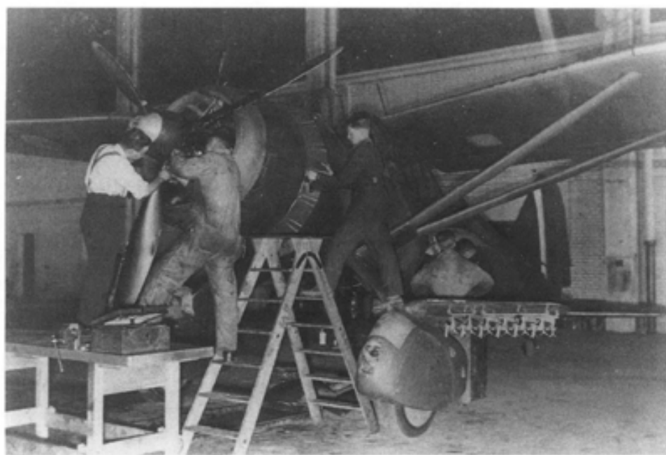
Fitters work on the engine of a Lysander of No 110 Squadron, RCAF (later No 400), in a hangar at Odiham in the autumn of 1940. The objects in the stub wing protruding from the undercarriage are light bomb racks. (PMR 93-296)
