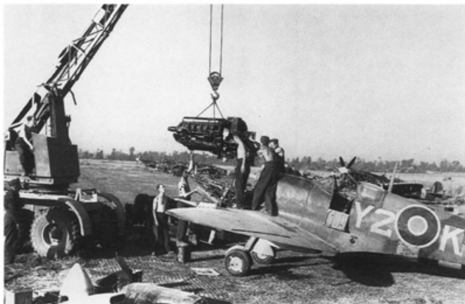
A No 442 Squadron Spitfire undergoes an engine change in August 1944. (PL 31363)
