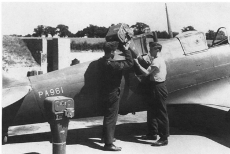
Groundcrew load an oblique camera into a Spitfire XI of No 400 Squadron in the autumn of 1944. (PL 40301)
