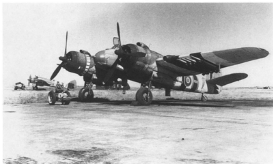
A Bristol Beaufighter Mark X of 404 Squadron with freshly painted invasion stripes in June 1944. The primary anti-ship weapon used by the Canadians was the 3-inch rocket with a 25-lb armour-piercing warhead launched from underwing rails. (PL 41049)
