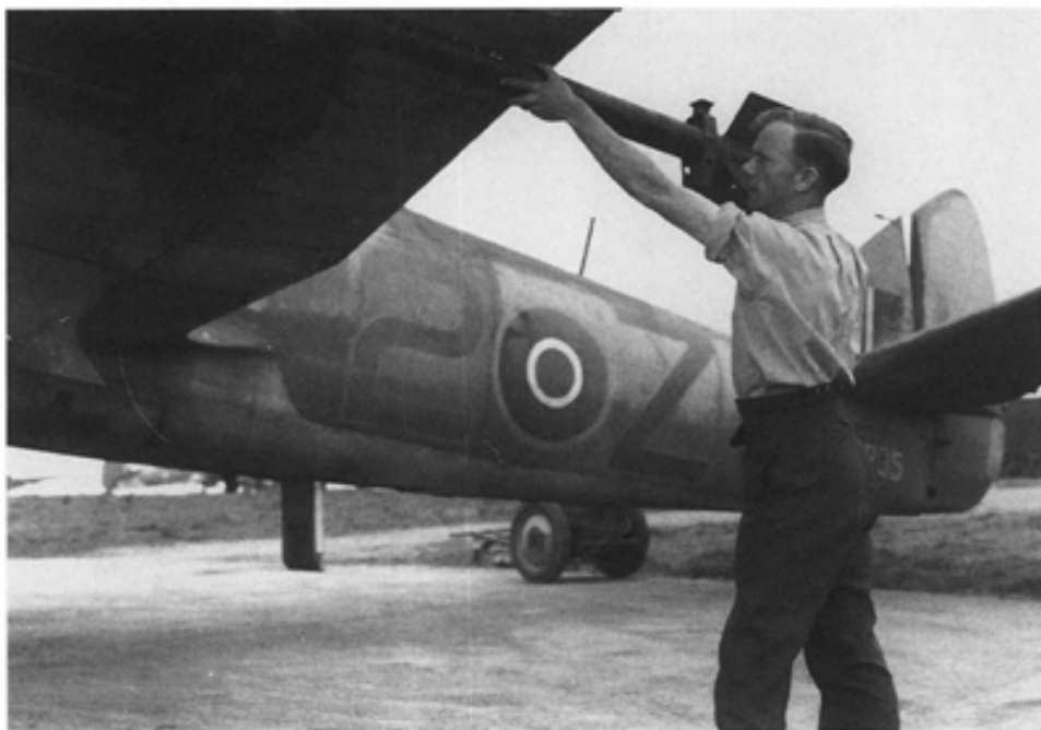
An armourer slides a 3-inch rocket onto the underwing rails of a Canadian Beaufighter. (PL 41007)
