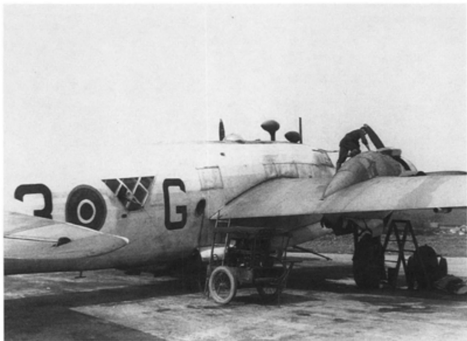
Servicing a Leigh Light Wellington. The beam gun position clearly shows the aircraft's geodetic lattice-work construction that made it such a rugged machine, capable of withstanding great punishment. (PL 40927)
