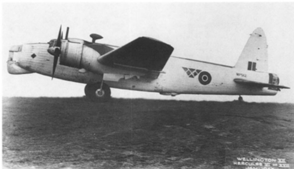
A Leigh Light-equipped Vickers Wellington Mark XII similar to those used by No 407 Squadron. The retracted Leigh Light is visible on the underside of the fuselage just behind the wing, while the ASV III radar is located in the dome under the nose. (RE 19876-11)
