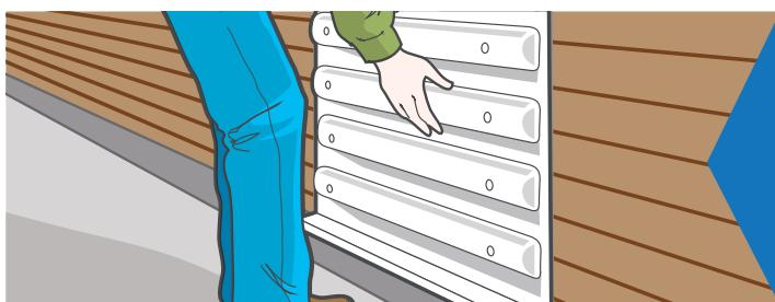
Install flood shields/barriers for basement windows and doors.
