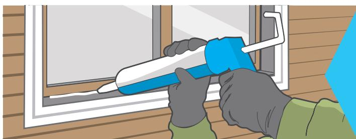
Put sealant around basement windows and beneath ground-level doors.
